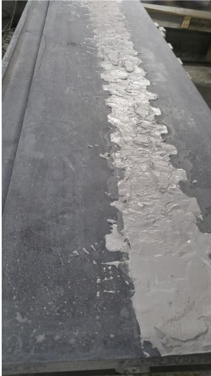
We purposefully over-fill the negatives. When the concrete cures and shrinks, just the right amount of material will remain. If it looked perfect when wet, it would be full of holes when dried.
