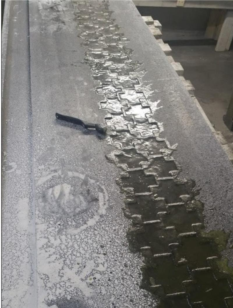
*This bar top has already been ground flat. Note the pattern of tessellated crosses. After applying acid to the negative spaces, Alyre scrubbed every single cross with a small brush, to make sure acid reached all corners.*
